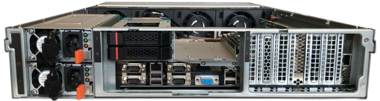
eMAG Lenovo Server Rear View
