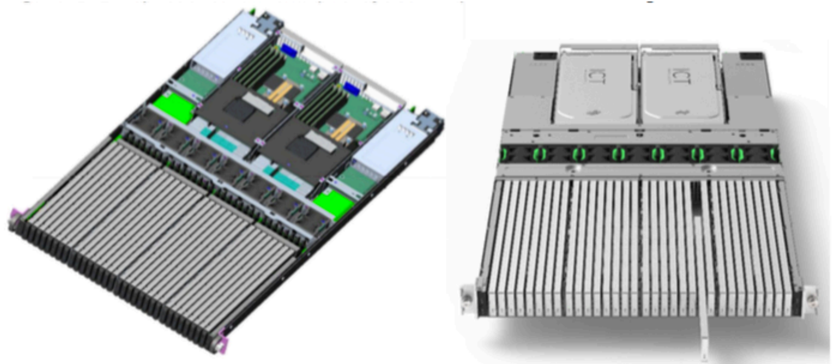
Example system with 1U Long cards
